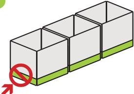
Containers should be stacked (open or collapsed) with same sides in alignment. Each container's feet should interlock with the lid or container below it.
