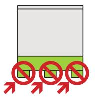
When handling "hot" bins (>140° F.), pick from the 48" side. Caution: Forks will protrude past the opposite side and care should be used to prevent damage adjacent bins. Fork stops are recommended. **Do not short fork.**
