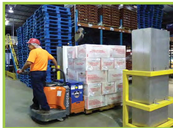
A pallet of 25 fully-loaded corrugated plastic boxes passes through an RFID scanning portal, which tracks their voyage into the distribution channel.
