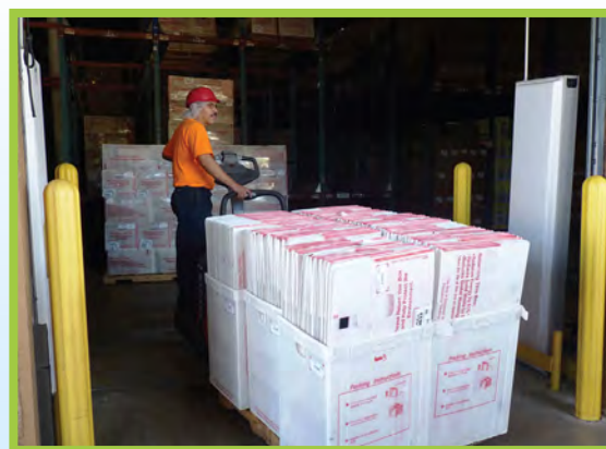
Flattened down and secured in purpose-built corrugated plastic tubs, 150 boxes return to the production facility on the same sized pallet, delivering an impressive return ratio of 6 to 1.
